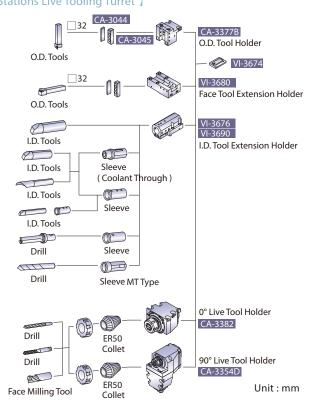
GS-8000 Series Construction Spindle Turre
