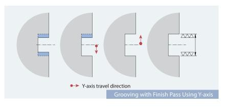
Grooving with Y-axis control produces grooves with higher accuracy.
