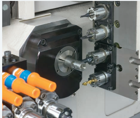
▶ Main & Sub-spindle simultaneous drilling and tapping
