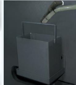
Built-in lub. oil collection system
